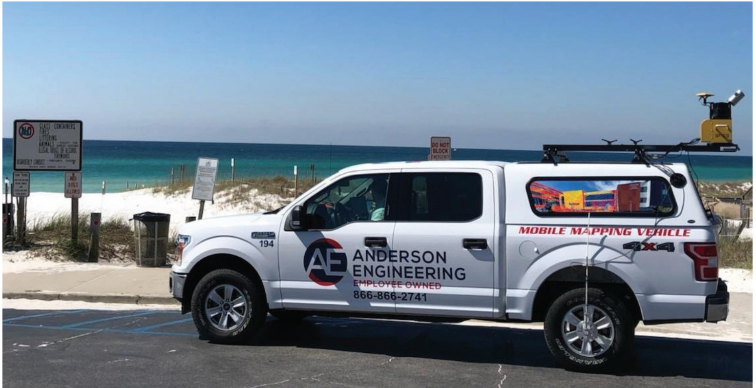
Example of a Mobile LiDAR unit vehicle setup
